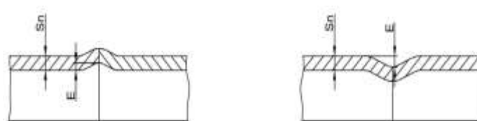
Fig.3 Schematic Diagram of Axial Angular Height of Circumferential Butt Weld
