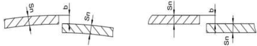
Fig. 1. Misalignment of Longitudinal Seams and Circumferential Seams
