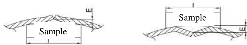
Fig.2 Height of Circumferential Corner Angle of Longitudinal Seams
